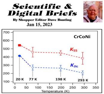
KJIc represents the crack-initiation toughness and Kss the crack-growth toughness. The KJIc and Kss values for the CrCoNi alloy are believed to be among the highest toughnesses ever reported. Image: School of Physics, University of Bristol
